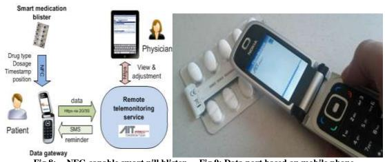
Fig 8: NFC-capable smart pill blister Fig 9: Data port based on mobile phone
