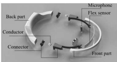
Fig 5: Neck Worn Sensor Designed by Wu et al.<sup>13</sup>
